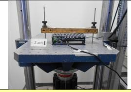
11. Mechanical Shock Test: -Z axis
