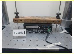
10. Mechanical Shock Test: +Z axis
